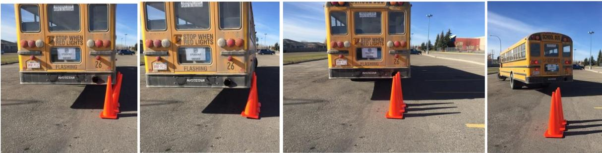
The Mirror Grid Activity- this activity helps school bus operators to correctly adjust their mirrors so they have optimum view around the bus and to minimize blind spots.
