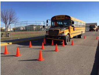
The Forward and Backward Serpentine Activity- this gets drivers really used to and comfortable with how the bus maneuvers and handles prior to heading out on the road. Drivers must weave between the cones forwards and backwards keeping the back tire no more than one foot from the cone as they pass it.
